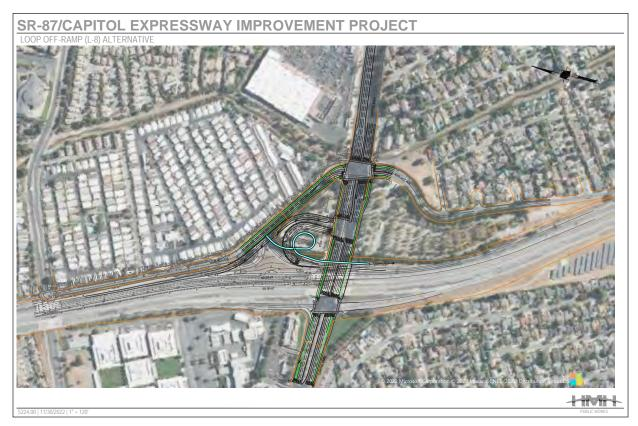
Figure 3.8 Overcrossing with Loop Off-Ramp Alternative
