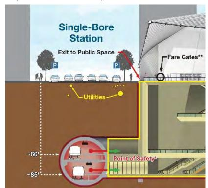
Vertical circulation elements such as stairs, elevators, and escalators in the stations would be in a similar configuration as other BART underground stations.
