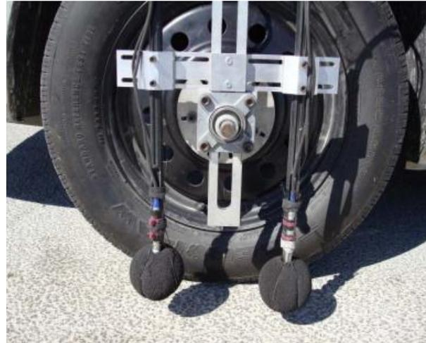
Figure 5-7: On Board Sound Intensity Measurement
